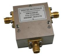
F2612-0300-67 is a single junction coaxial circulator with SMA female coaxial connectors operating in the frequency range from 2.0 to 4.0GHz and offers 0.35dB typical insertion loss and 19dB typical reverse isolation,. The power rating of this device is 50 watts CW power.
