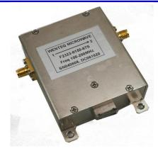
F2323-0150-67S is a single junction lumped element type isolator with SMA female coaxial connectors operating in the frequency range from 100 to 200MHz. It offers 1.0dB maximum insertion loss and 15dB minimum reverse isolation. The coaxial isolator can handle 20 watts of forward CW power and 10 watts of reverse power.
