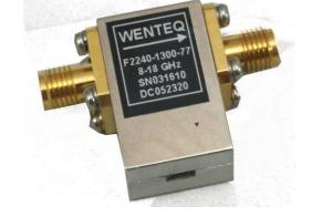
F2240-1300-77 is a single junction coaxial isolator with SMA female coaxial connectors operating in the frequency range from 8.0GHz to 18.0GHz and offers 0.8dB typical insertion loss and 16dB typical reverse isolation. The coaxial isolator can handle 10 watts of forward CW power and 1 watts of reverse power.
