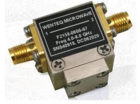
F2158-0600-67 is a single junction coaxial isolator with SMA female coaxial connectors operating in the frequency range from 4.0GHz to 8.0GHz and offers 0.6dB maximum insertion loss and 18dB minimum reverse isolation. The coaxial isolator can handle 10 watts of forward CW power and 1 watts of reverse termination power.
