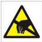
**WARNING:** This device is electrostatic sensitive, please observe precautions for safe handling of this amplifier.
